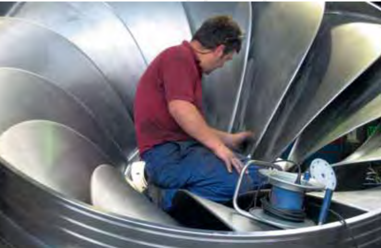
Being aware of the importance of the welding, each Francis runner is consciously assembled by qualified personnel.
